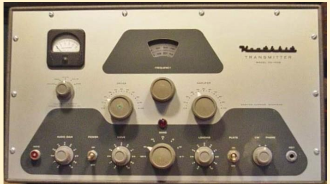
Fig. C Heathkit DX-100, 100 Watt AM/CW transmitter
